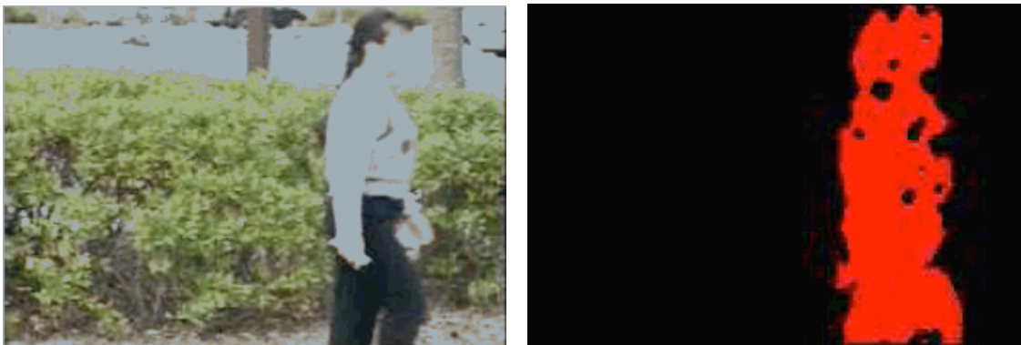
Figure 6: A figure showing the background subtraction technique used in conjunction with a complementary technique (salient motion) developed by researchers at IBM applied to a human being moving in a camera frame 324 . Note that the pixels pertaining to the human being in the foreground have been identified and made red in the second image.
